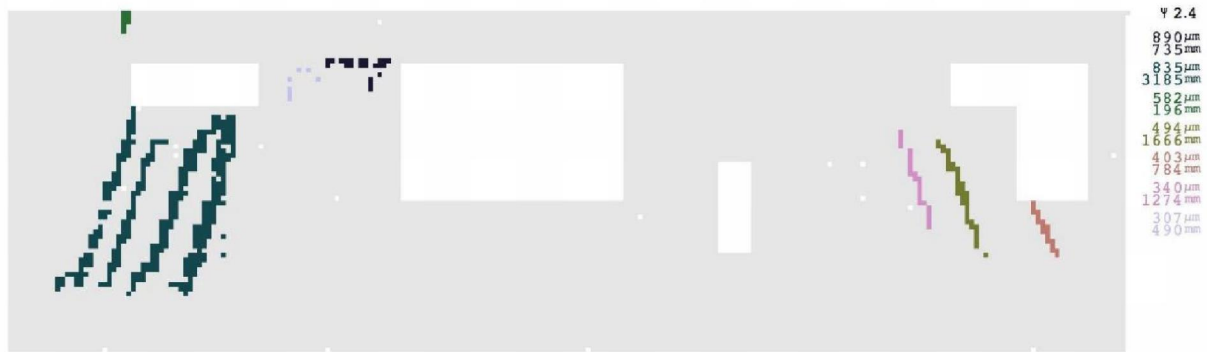
Figure H9. Crack pattern of Façade 4, subjected to hogging SH2 (left) and sagging SS4 (right). Cracks at DS2.
