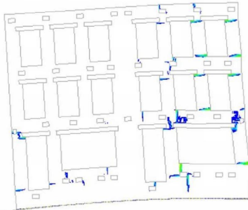
Model EMM – f_{tx} = 0.10 MPa, c = 0.03 MPa
