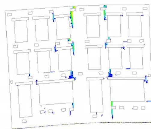
Model EMM – f_{tx} = 0.15 MPa, c = 0.03 MPa
