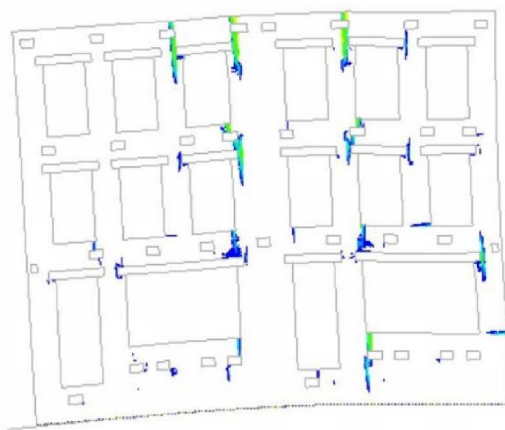
Model EMM – f_{tx} = 0.10 MPa, c = 0.03 MPa
