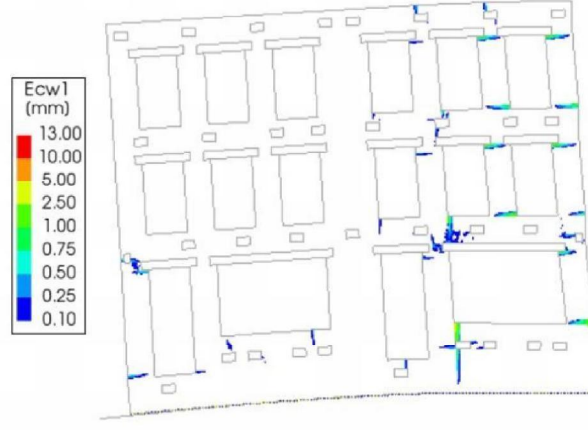
Model EMM – f_{tx} = 0.15 MPa, c = 0.03 MPa
